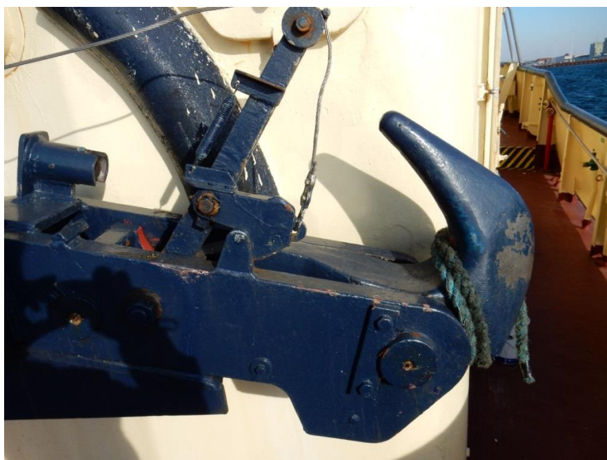
Figure 8. Hook with emergency release on board BONDEN.
