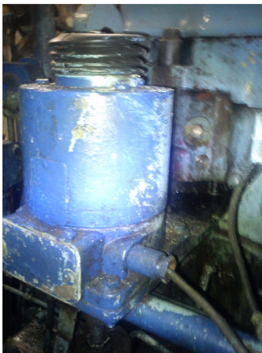
Main engine emergency stop unit
