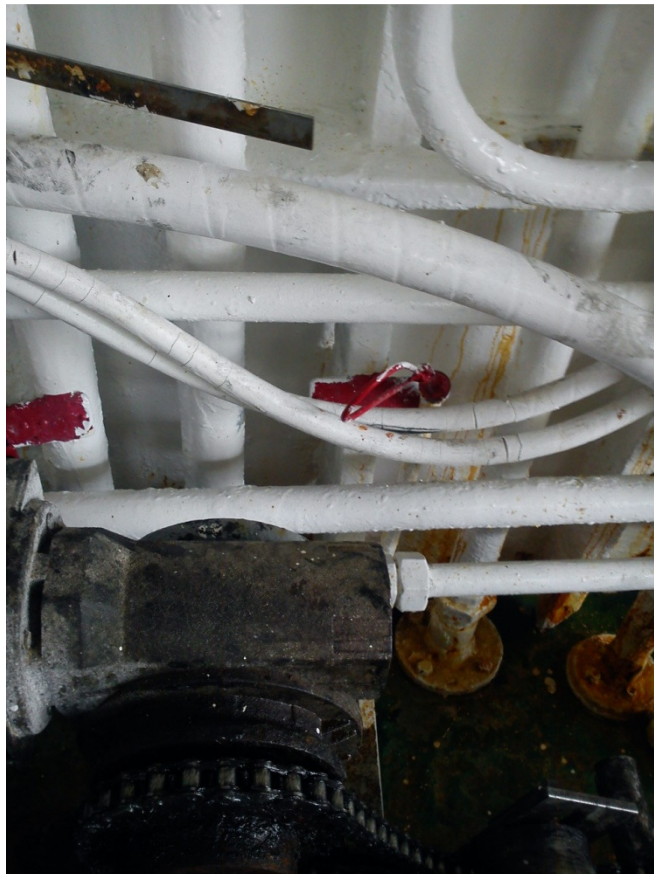
Remote for quick closing valve day tank. Located main deck SB.
